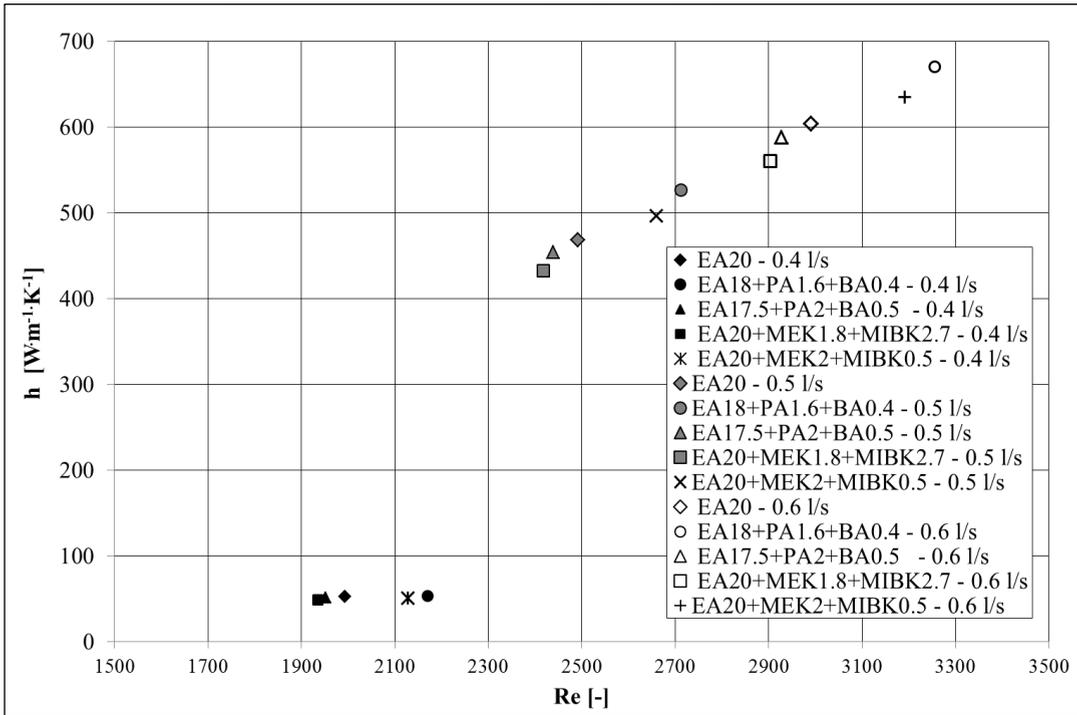
Fig. 5. Convection heat transfer coefficient vs Re number for different flow rates in PE40 x 2.4 mm U-pipe BHE at  $T = -5\text{ }^\circ\text{C}$ .
