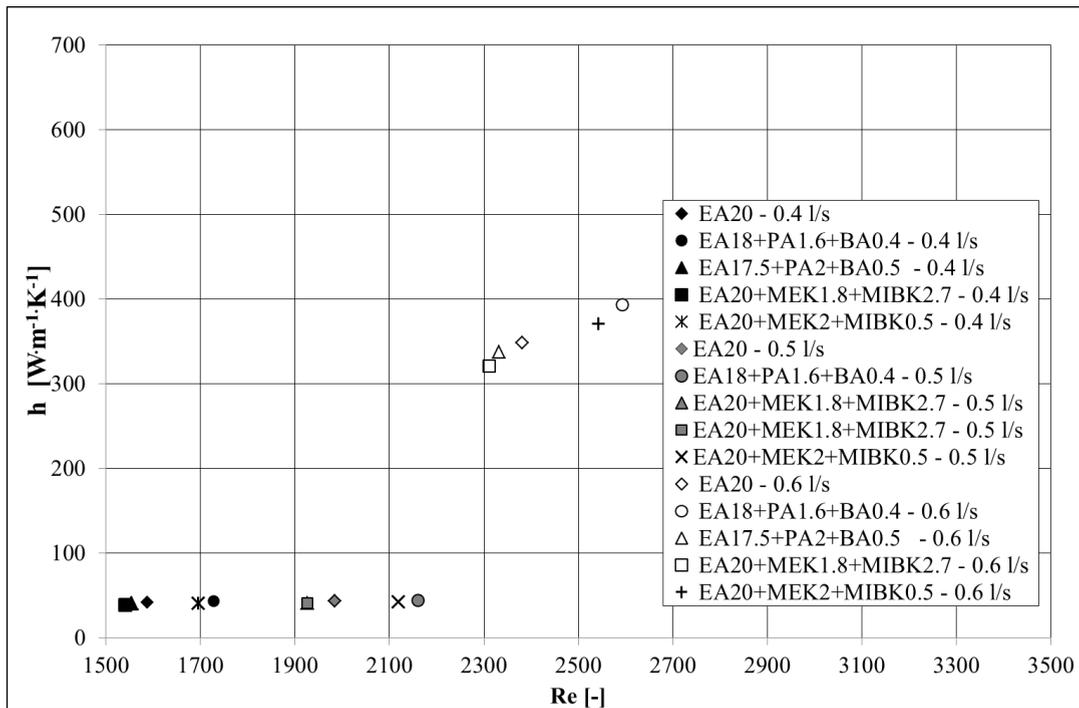
Fig. 6. Convection heat transfer coefficient vs Re number for different flow rates in PE50 x 2.9 mm U-pipe BHE at  $T = -5\text{ }^\circ\text{C}$ .
