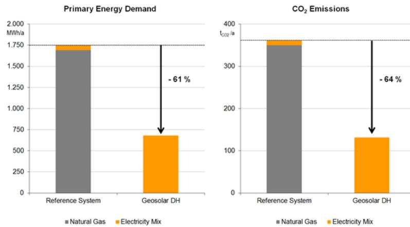
Figure 6: Primary energy demand (left) and CO<sub>2</sub> emissions (right) of the geosolar and the reference heat supply system
