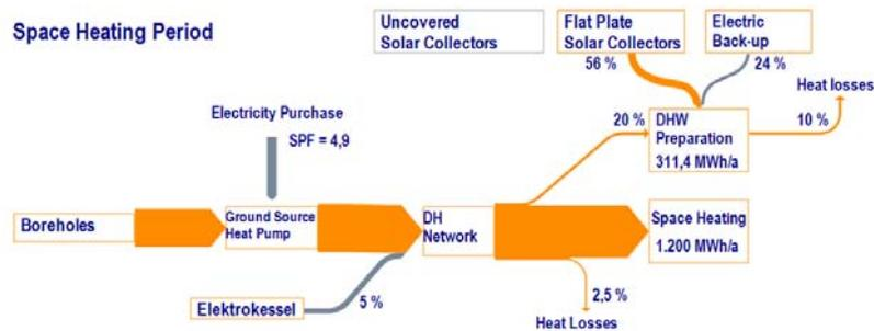
Figure 4: Energy flows during the heating period (Oct-Apr)
