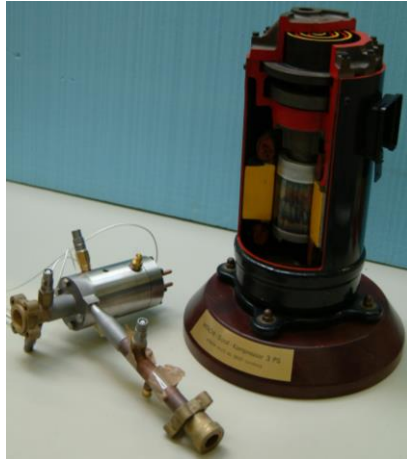
Figure 3: Comparison of the single-stage proof-of-concept radial compressor on gas-lubricated bearings and an equivalent scroll compressor [12]
