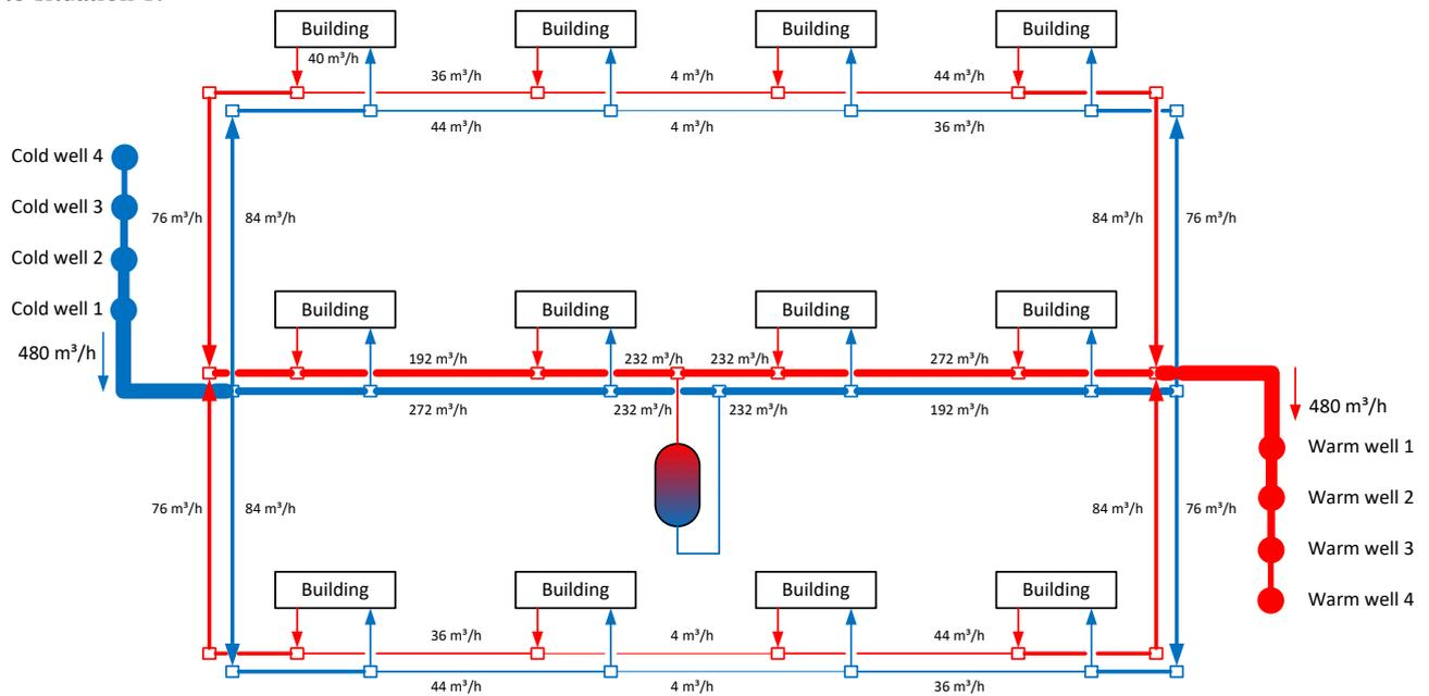
Fig. 6. Situation 1: DATES well locations alongside the loop
