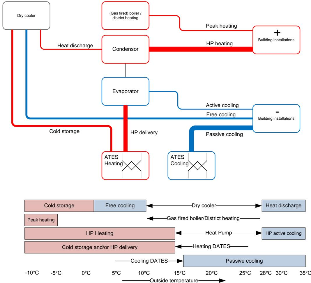
Fig. 1. Standard ATES/HP configuration and indication of operational mode depending on outside temperature
