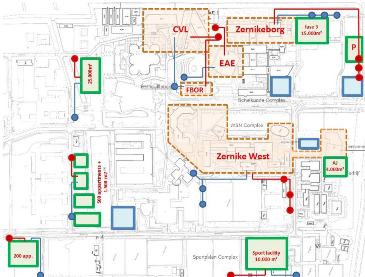
Fig. 3. Individual ATES system per building, Zernike Campus University of Groningen
