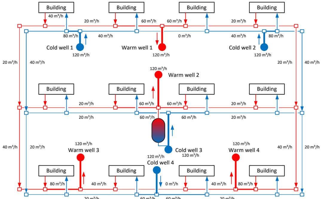
Fig. 7. Situation 2: DATES well locations within the loop
