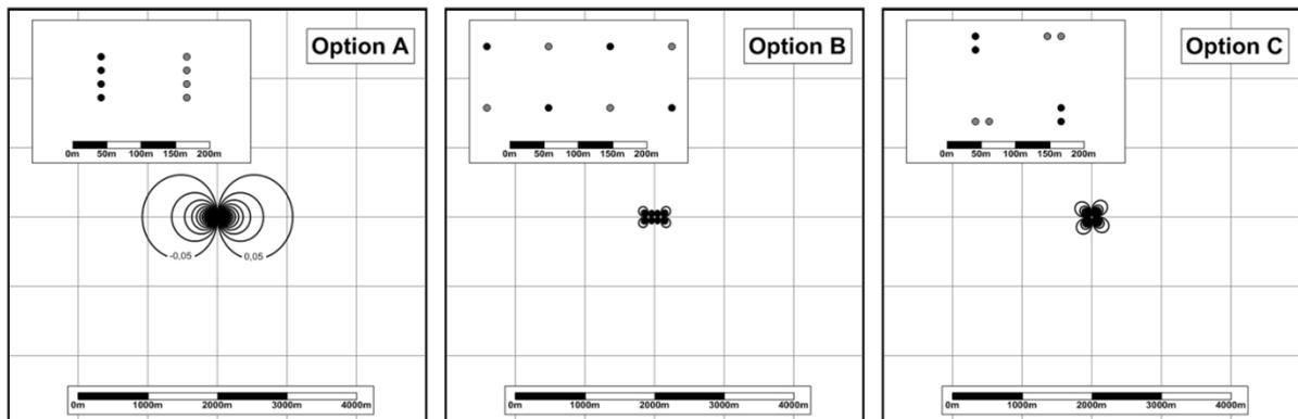
Fig. 5. Calculated drawdown in the aquifer in three situations with different well field layout and equal numbers of wells and total flow rate[5]
