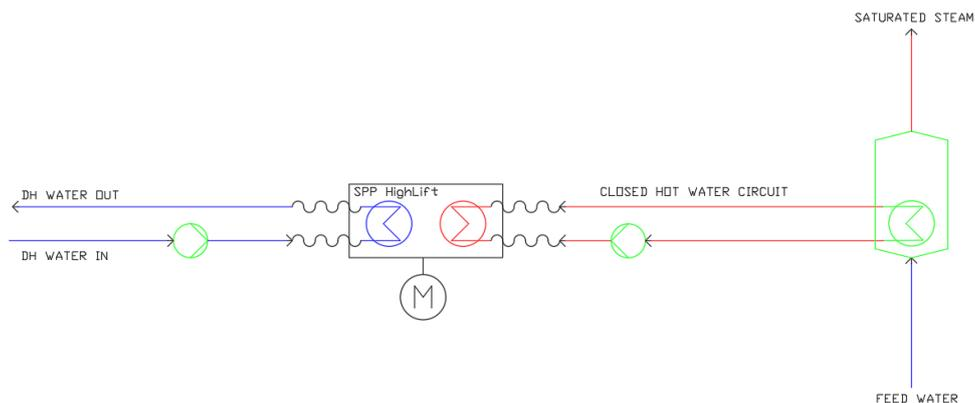
Fig. 2. Simplified P&ID of the installation of one heat pump. The closed hot water circuit heats the feedwater to the saturation temperature and evaporates the water in a plate and shell heat exchanger.
