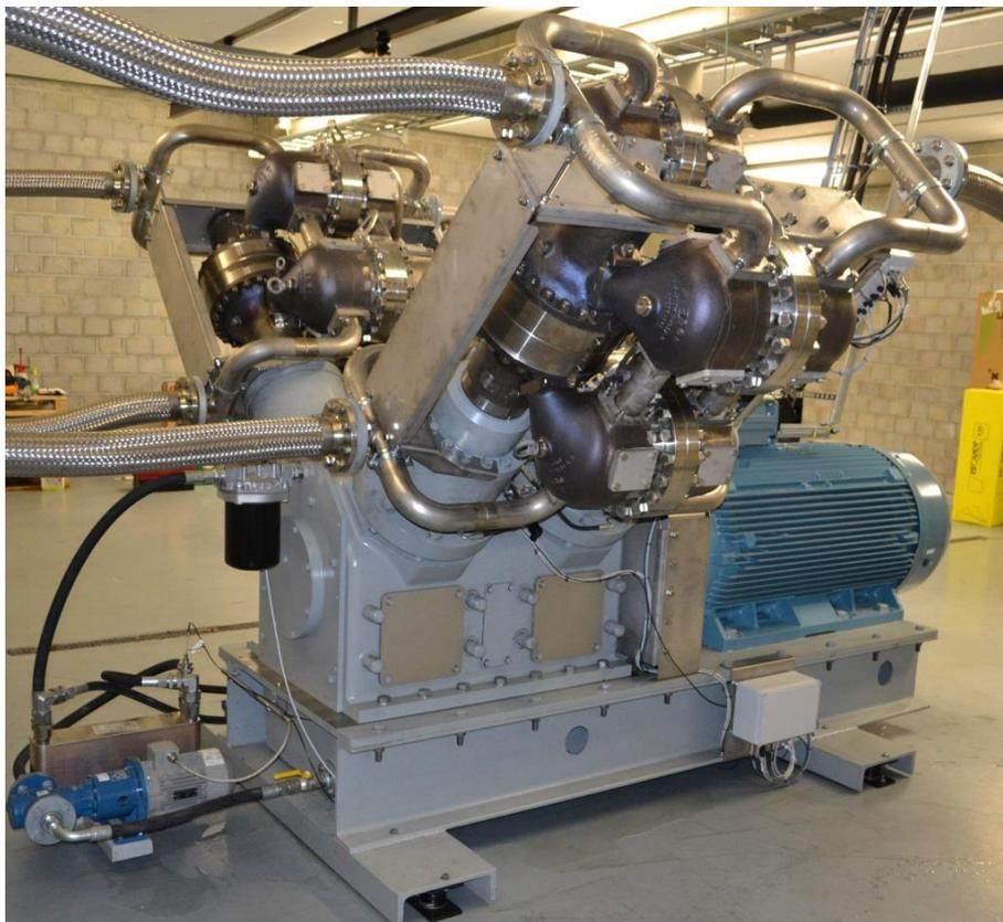
Fig. 1. Photo of the SPP HighLift heat pump (SPP 4-106C) at Lerum Fabrikker AS, Norway. The heat pump at this site generates steam at 6 bar<sub>g</sub> in a flash tank using waste heat from cooling compressors as the heat source.
