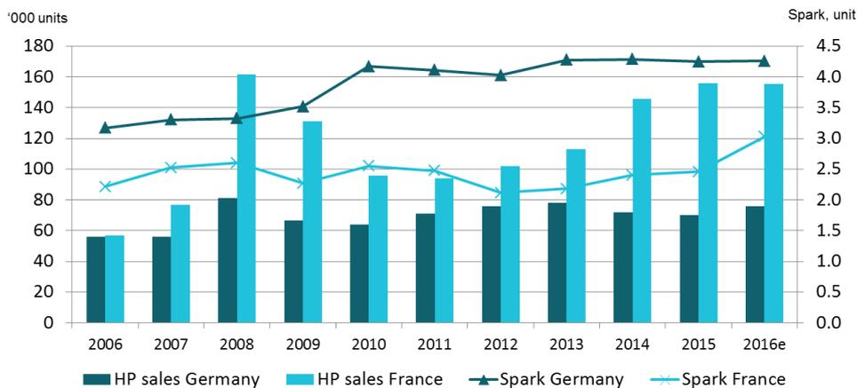
Figure 2: Sales of hydronic heat pumps in Germany and France against the electricity / gas price ratio, units, 2006 – 2016(e) (Source: BSRIA)
